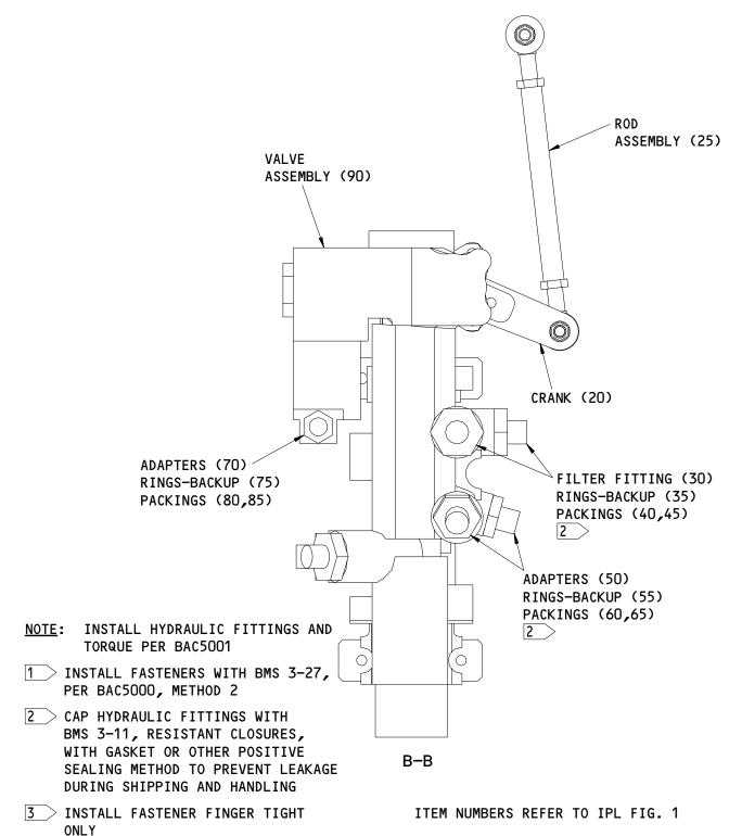
Brake Metering Valve Assembly Figure 701 (Sheet 3)
