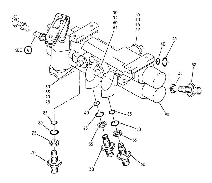
Brake Metering Valve Assembly Figure 1 (Sheet 1)
