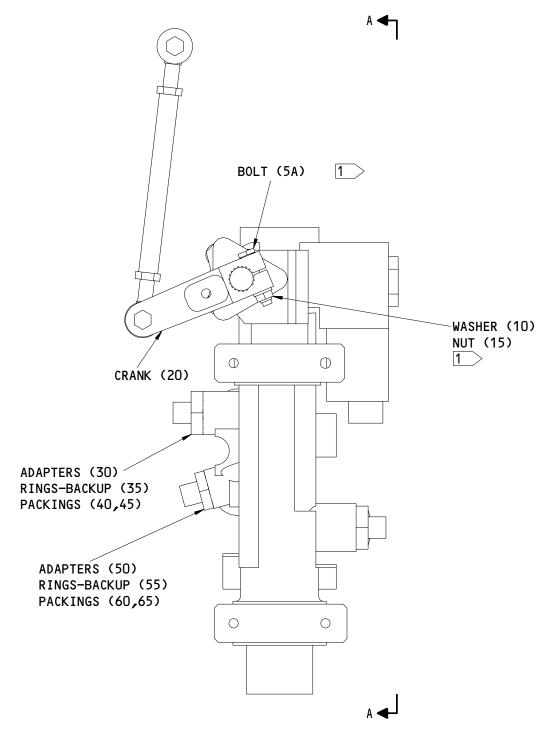
Brake Metering Valve Assembly Figure 701 (Sheet 1)
