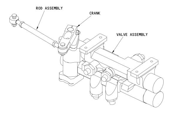
Brake Assembly Metering Valve Figure 1
