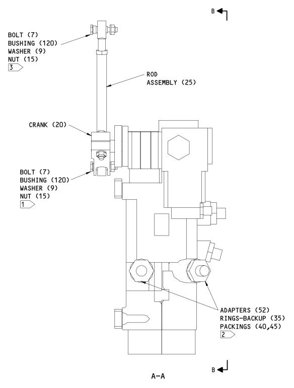
Brake Metering Valve Assembly Figure 701 (Sheet 2)
